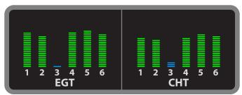
There's no combustion in that cylinder, so complete injector blockage is likely. The roughness is caused by one cylinder producing no power. You could try full rich and boost to clear it in some engines. This pattern could also be no compression due to a stuck valve, which would be even more serious.
