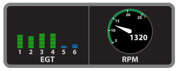
Check for blow-by in the cylinders with the lower EGT(s) by conducting a compression test.
