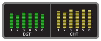
This could be normal on a high density altitude summer day, if it's minor. However, advanced timing could cause this, which is why you should look for this behavior during runup (page 29). The early spark is creating greater heat during combustion. This would be more likely after engine work where the magnetos were touched. If the timing is seriously advanced, it's possible EGTs could be higher than normal, but this would be so far advanced that detonation may become an issue.
