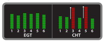
Because this may be detonation, reduce power if it's at all safe to do so. Increase cooling with full rich mixture (which will also help suppress detonation), and open cowl flaps. If the CHTs reached the danger zone, you should consider diverting for landing now. Note that EGTs may remain normal throughout.
