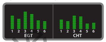
This is common with poor fuel distribution in large, six-cylinder carbureted engines. However, dirty injectors or multiple fouled spark plugs can cause this pattern.
