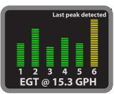
You'd only see this if attempting LOP operations, because you'd need all cylinders to pass through peak EGT (or have the engine go rough by the time all cylinders should have passed through peak EGT).
