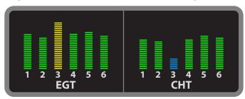
There's low power generated in that cold cylinder, which could be a badly clogged injector or fouling of both spark plugs. You probably have at least somewhat rough operations as well.
