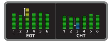
While this could be one slowly failing plug or wire, if the slow rise is over many flights, it's more likely an exhaust valve that's burned or not seating well. Again, heat energy is escaping the cylinder, so the EGT is higher but CHT is normal or low.
