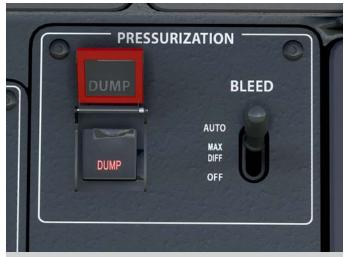
*Decompression is an additional tool in a pressurized cabin for clearing the air.*
