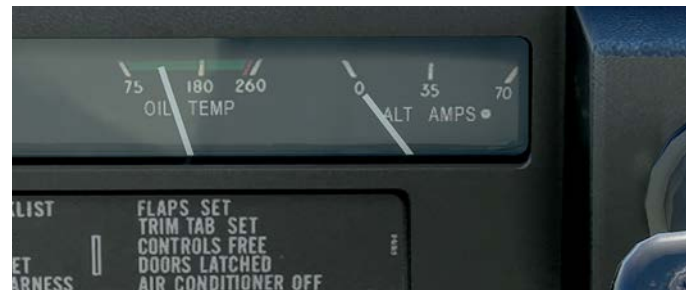
A loadmeter (as in older Pipers like this one) shows the output of the alternator. When the alternator fails, the loadmeter reads zero.
