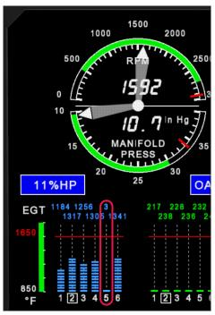
If you have electronic ignition replacing a magneto (page 119) or a Rotax engine, the ignition checks obviously change. Dual electric systems with a carbureted Rotax typically do show a drop when running on one module. Electric engine controls such as the injected Rotax or some aftermarket magneto replacements often show no drop. However, they will show an error (hopefully with a code) if there's a problem.
