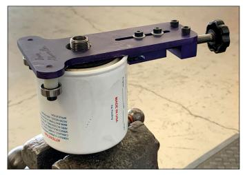
Once you cut open the filter (above), you can remove the outer case and see the oil filter element (upper right). Oil passes through the filter element from the outside to the inside, so you'll see debris on the outside of the pleats. To better see between them, cut out the filter material with a knife, so you can spread it out flat on a table (right).
