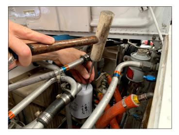
Oil can get trapped inside the oil filter and make a mess when you remove it. This is more of a problem when the filter is up high on the engine. You can punch a small hole in the top of the filter with
