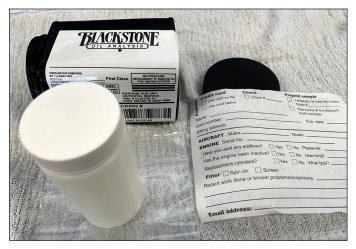
Sort of a like a urine sample, you catch the oil middrain. The catch cup comes with the oil sample kit, along with instructions for sending it to the lab.
