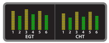
In this case, there's more heat coming out the exhaust, but there's also more heat generated inside the cylinder during combustion (hence the high CHT), so there must be significantly more heat generated in this cylinder.
