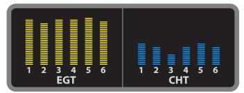
This could be retarded timing or failure of one magneto. The airborne ignition check could clarify. Know that if a mag has failed, the engine may cease to run when switching to that mag.
