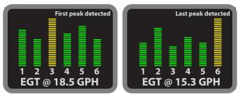
You'd only see this if attempting LOP operations, because you'd need all cylinders to pass through peak EGT (or have the engine go rough by the time all cylinders should have passed through peak EGT).
