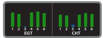
There's no combustion in that cylinder, so complete injector blockage is likely. The roughness is caused by one cylinder producing no power. You could try full rich and boost to clear it in some engines. This pattern could also be no compression due to a stuck valve, which would be even more serious.
