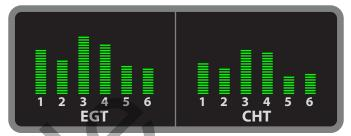
This is common with poor fuel distribution in large, six-cylinder carbureted engines. However, dirty injectors or multiple fouled spark plugs can cause this pattern.
