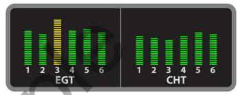
You have poor combustion in that cylinder. The likely culprits are a fouled spark plug, or failure of the spark plug or wire. Here's a way to think about it that's a bit simplistic, but can be helpful. You could say that heat going out the exhaust is energy from combustion that's not spinning the prop for you.
