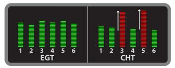
Because this may be detonation, reduce power if it's at all safe to do so. Increase cooling with full rich mixture (which will also help suppress detonation), and open cowl flaps. If the CHTs reached the danger zone, you should consider diverting for landing now. Note that EGTs may remain normal throughout.
