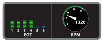
Check for blow-by in the cylinders with the lower EGT(s) by conducting a compression test.
