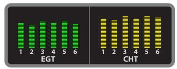
This could be normal on a high density altitude summer day, if it's minor. However, advanced timing could cause this, which is why you should look for this behavior during runup (page 29). The early spark is creating greater heat during combustion. This would be more likely after engine work where the magnetos were touched. If the timing is seriously advanced, it's possible EGTs could be higher than normal, but this would be so far advanced that detonation may become an issue.
