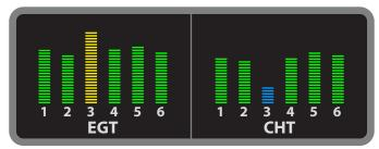
There's low power generated in that cold cylinder, which could be a badly clogged injector or fouling of both spark plugs. You probably have at least somewhat rough operations as well.
