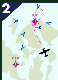
2 Overfly the airport, descend once north, and return for a 45 to right downwind Runway 34.
