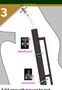
Add enough power to get rudder authority and straighten out. Then, power up all the way and go around.
